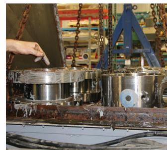
Valve is flushed, cleaned and inspected
