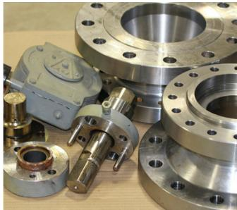
Metal parts prepped and ready for the dip tank
