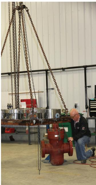
Damaged parts are discarded and replaced, all soft goods are replaced
