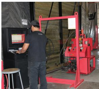
Valve is reassembled and hydro-tested
