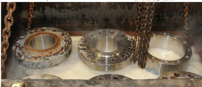
Metal parts are stripped of any petroleum products and paint
