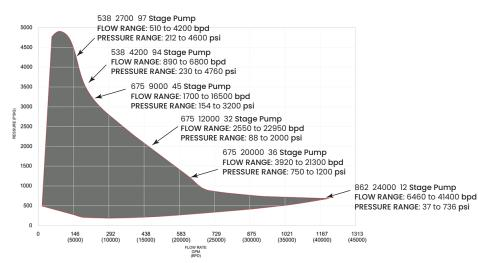
A **single** Flex Flow HPS can be run with the results as shown above. Multiple systems may be run in parallel or in series and are easily configured in the field. All combinations fit a common skid. VFD and PLC controls offer additional flow and pressure flexibility.
