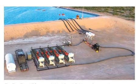
The Flex Flow HPS system is ideal for all fluid transfer operations, including storage and capacity applications, pump replacement/ backup, brine and hydrocarbon transfer, and brine disposal.
