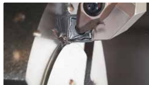
Machine Tools – rough turning cast iron
